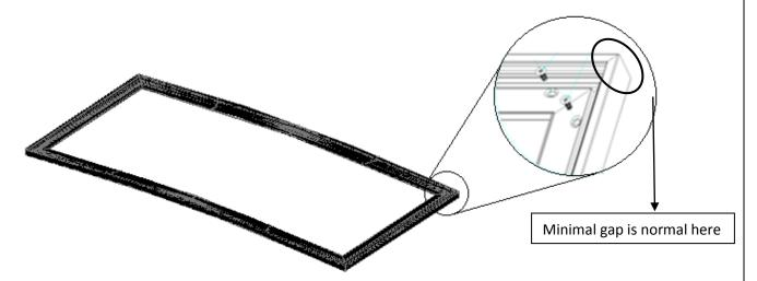
3. Layout the **Screen Material** and **Tension Rods** on a clean and dry surface. Then, gently roll out the screen material over the back of the fixed frame.
