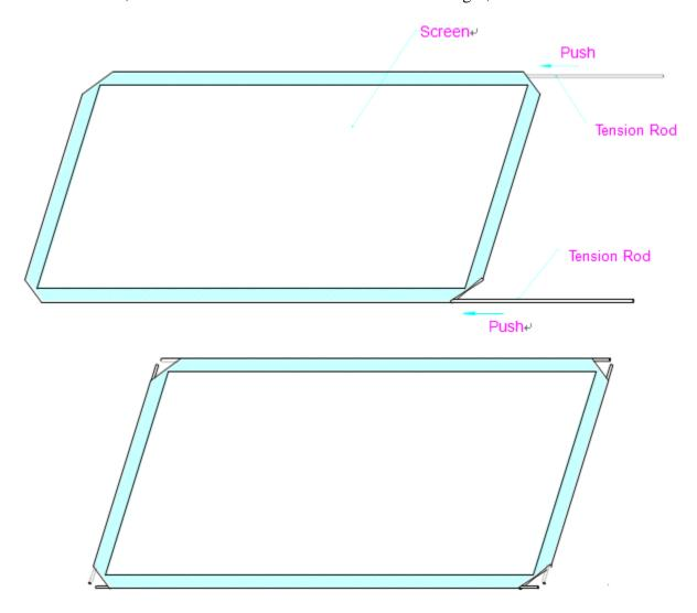
5. Slip the screen tension rods into the grooves running along the back of the frame. Clip on the **Fix Plates** to the back of the frame to secure the rods into place forming a tight and flat surface. See **Attaching the Fix Plates** section below for details.
