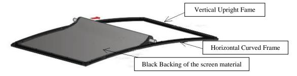
4. Insert **Tension Rods** through the sleeves. The longer rods are used on the horizontal edges of the screen material, and the shorter rods are used on the vertical edges, as seen below.
