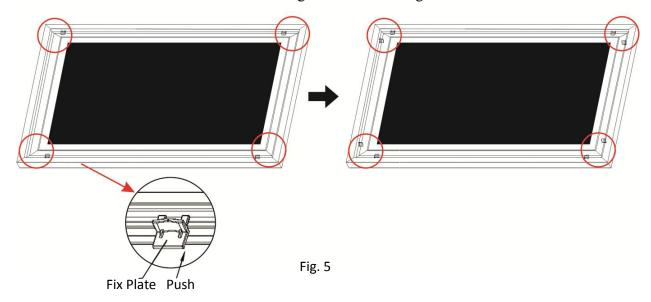
4. Attach the fix plates starting from the ends and moving towards the center as shown in the diagram below to create an evenly tensioned surface.
