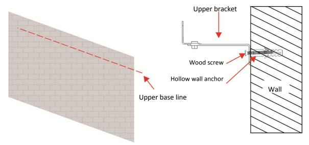
3. Draw a lower base line according to the data F of P10 diagram and the upper base line, and then make a hole on the wall according to the screw hole location for the lower bracket, then insert the anchor and tighten the lower bracket with the provided screw.
