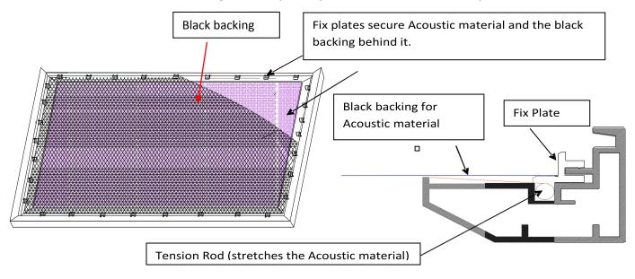
Interval markings reveal the best points for inserting the fix plates (Fig. 1). The prongs on the fix plates insert to the lip on the back of the frame creating a friction hold that will firmly keep the material and black backing in place (Fig. 2-3). After the material has been installed, the backing will lie over the back of the white (Acoustic) material and then be held in place by the Velcro on the fix plates (Fig 4).
