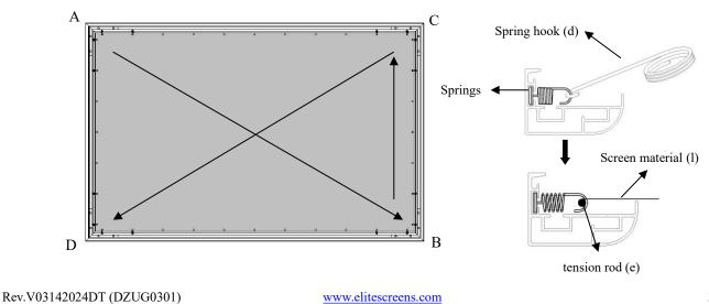
5. Next, attach a spring in each center point locations (1), then out of the center location (2), and finalize the installation with the remaining springs.
