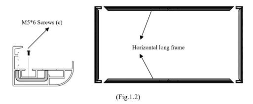
5. Join all four frame parts together following the steps shown below. (Fig.1.3) Note: When assembled, please push simultaneously the two ends of the long frames.
