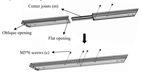
Note: a. Two ½ horizontal long frames should be assembled for a screen. b. Do not tighten the screws completely until all frame pieces have been assembled correctly.
