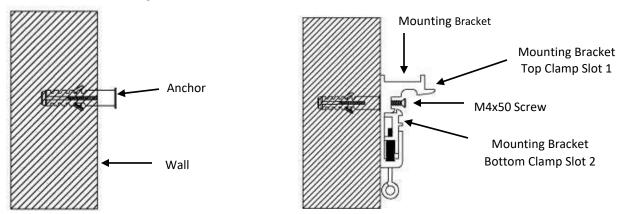
3. Insert and attach the *Top Case Slot A* to the *Top Clamp Slot 1*, then secure it by pushing and clicking it in the *Bottom Clamp Slot 2* to the *Bottom Case Slot B*. Make sure the case slots are securely attached to the mounting brackets.
