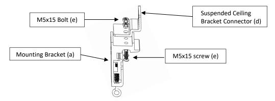
3. Insert chains (not included) through the loopholes of the Suspended Ceiling Bracket Connector (d).
