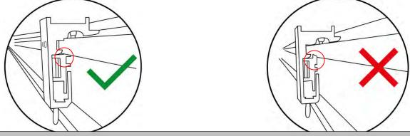
**CAUTION**: THE WALL BRACKET MUST BE SECURELY LATCHED IN THE CASE SLOTS TO PREVENT THE CASE FROM FALLING OFF.
