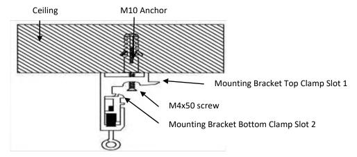
3. Insert and attach the *Top Case Slot A* to the *Top Clamp Slot 1*, then secure it by pushing and clicking it in the *Bottom Case Slot B* to the *Bottom Clamp Slot 2*. Make sure the case slots are securely attached to the mounting brackets.
